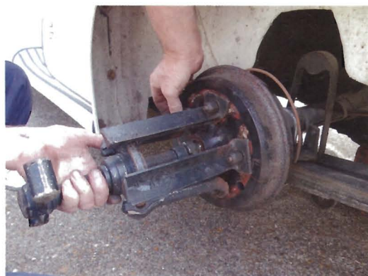
Drive shaft breakages are said to be common; needs a puller too
