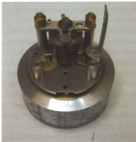
The coil removed ready to remove the input terminal for modification
