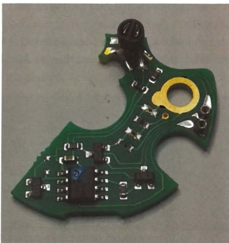
The circuit board showing the controller (bottom centre)
