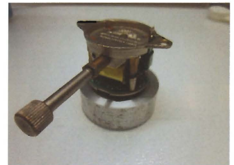
The finished clock with kit fitted ready for refitting into the Rev Counter.
