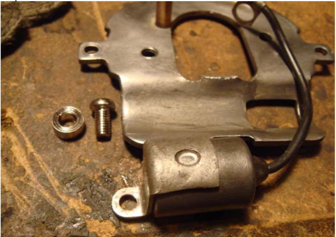
5. Drill and tap a 4mm hole for a standard 4mm machine screw. The screw will need to be long enough to just come through the other side of the base plate when you have a shake proof washer between the head of the screw and the condenser.
