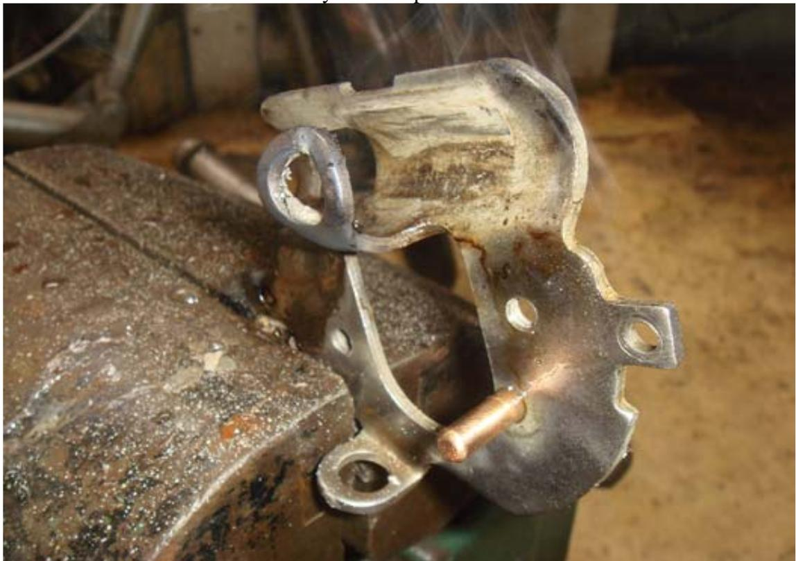
3. Discard the old condenser and saw off the hooked leg that held the condenser in place.
