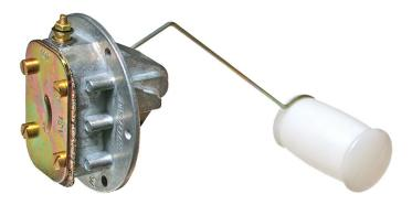
To perform these tests, you may need to drain the fuel tank before removing the sending unit from the tank. Remember that gasoline is a highly flammable liquid, and that the vapor in a gas tank is a highly explosive gas. Be very careful to keep open flames away, and not to do anything that could create a spark near the tank.
