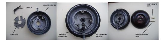
Two screws connecting the horn contacts to hub. Short brass screw to earth on hub body, long brass screw connects horn pigtail wire to horn power supply using an insulated sleeve and fibre washer with a nut. Access to this nut and bolt is only after clockwork mechanism has been removed.
