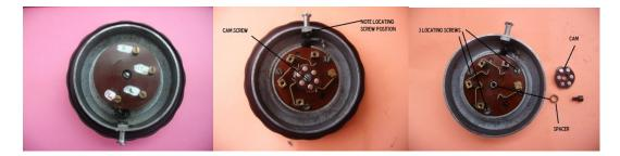
Remove centre screw to release contact cam assembly (note spacer under cam).
