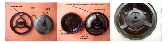
Further stripping of trafficator assembly shows spokes on moving outer switch and the pegs on the inner fixed hub of switch. ( have marked these with snopake just for reference). These must be lined up correctly or rotary outer part of switch will not move through full range.
