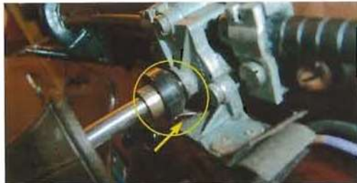
Here we can see the conic bakelite ring which (in pressed-in position) opened the contact tongue of the switch
