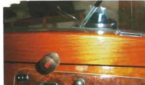
I marked the parking knobs to screw the wiper arms tight in the correct position
