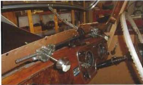
The wiper arrangement with driving links (wheel boxes) and the push and draw cable.
