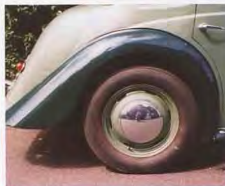
The easiest way to tell a YA from a YB is to look at the rear wings. The YA has bigger wheels, so the wing is shallower.
