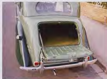
Check the boot lid and spare wheel cupboard for corrosion.
