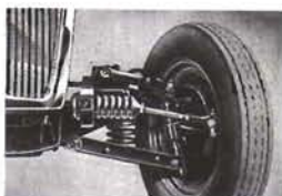
The arrangement of the independent front wheel suspension is simple, sturdy and mechanically light efficient.
