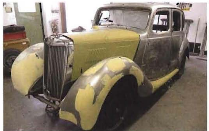
The body all repaired and ready for the first coat of primer.
