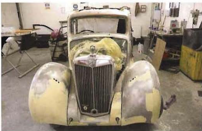
The repaired pillar all ready for painting.
