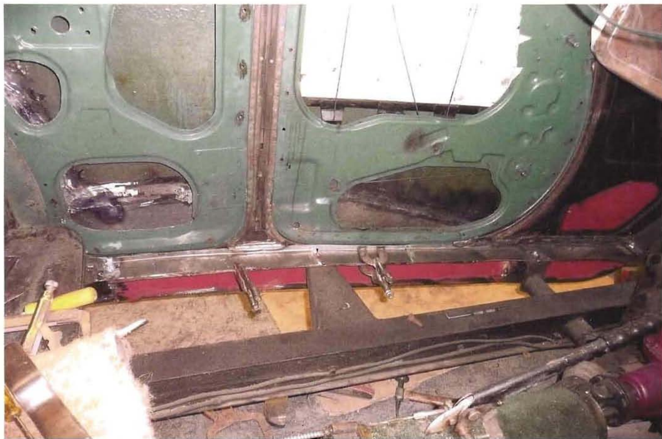
New near-side sill all fitted.
