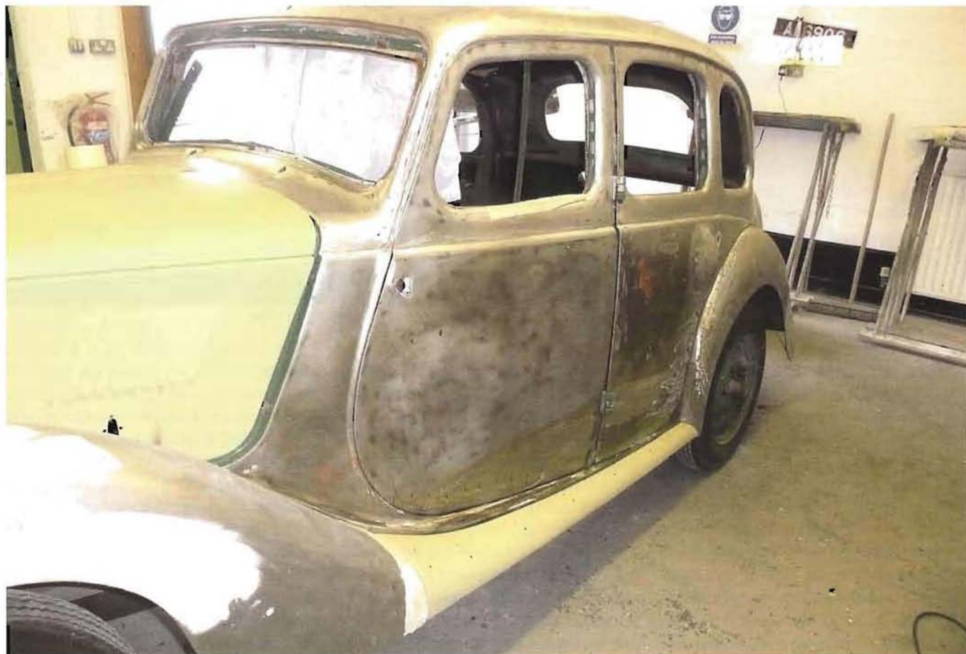
The professionally welded repair of the windscreen pillar.
