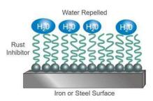
Some of these inhibitors are specific to protecting certain metals. An oil may contain several different corrosion inhibitors.
