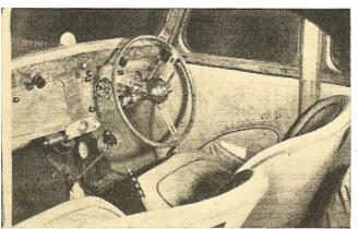
The neat appearance of the facia is marred by the untidy fitting of the controls for an American radio, of which the tone was very good. The glove locker has been removed, and the radio set itself occupies the entire space behind the lid. The car's handbook is in the door pocket.
