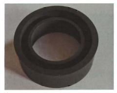
Inspired by the success of the ram seal I went through the same process with the pump shaft seal and we added them to our stock. Another part that was not readily available was the UNF 7/16th brass tube nut. All the copper tubes in the system are connected with brass compression fittings with olives, as in water plumbing systems.
