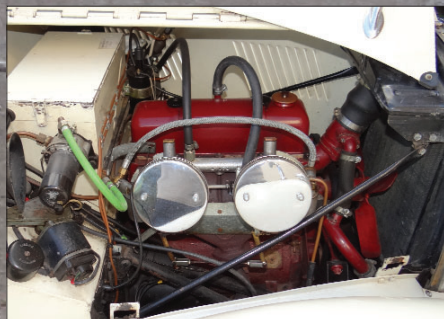
Engine Bay showing two carburetors
