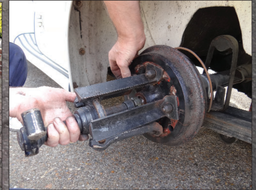
Five point puller needed to remove the rear hubs
