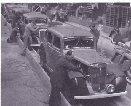
Almost ready for final inspection and the bonnet and headlights are fitted, the wiring connected up, petrol added to the tank and the car is then driven away for road test
