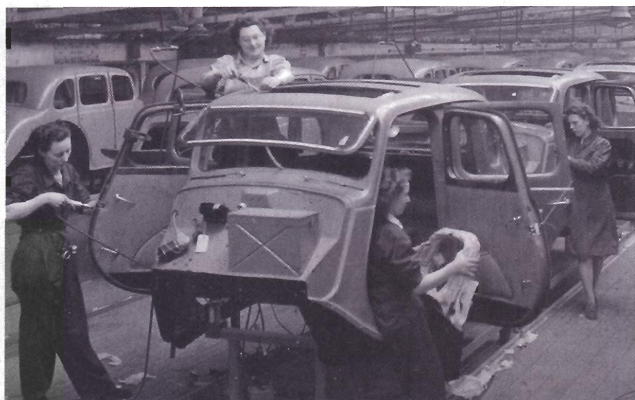
On the top floor of the assembly building the bodies were attached to trolleys so they could be rolled along this production line. Note the many female workers employed at the time
