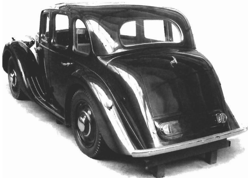
The original Y-type prototype, or MG Ten, at Cowley in 1939. It is just a mock up at this stage, with supporting blocks underneath, but the design was closely followed for production cars
