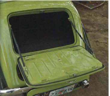
Similar in style to prewar Bentleys and Rolls-Royces, the YA saloon has a trunk lid that is hinged on the bottom and folds flat when opened. The spare tire hides behind the oval panel upon which the license plate and taillamps are fitted.
