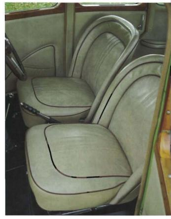
The interior features extensive use of wood, adjustable steering wheel, upright leathercovered seats, and the MG's signature octagonshaped instruments.
