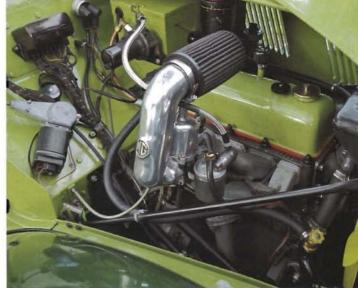
Inspired by his better performing MG race cars, George tweaked the YA's original XPAG OHV four-cylinder engine for added power. He installed a larger 11/2-inch H4 SU carb, higher-lift Crane camshaft, an alternator, K&N air filter, and had the engine block bored out to 1,350-cc.
