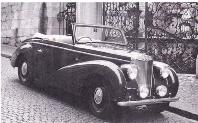
This two-seater Y-type was bodied in Switzerland for importers, J. H. Keller. The cut-away doors, dashboard and weather equipment closely resembled those fitted to the contemporary TC.
