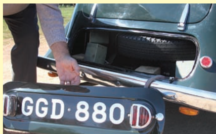
The spare wheel lives in its own compartment underneath the boot.
