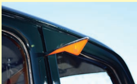
Original trafficators work, but have been supplemented with flashing lights.
