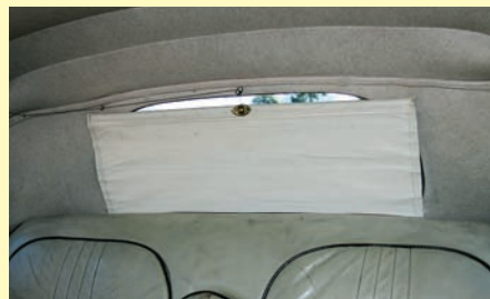
Bruce's Y-Type has a rear blind that can be raised and lowered by the driver.
