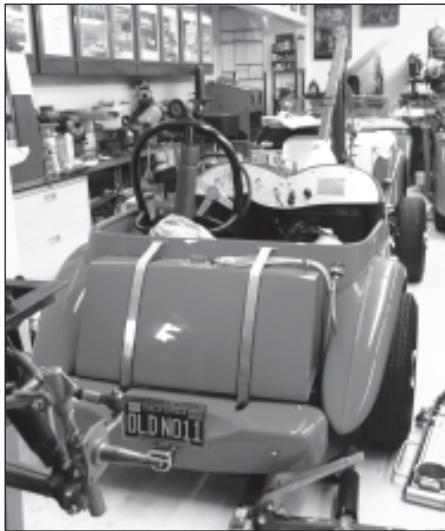
Above and below: 1950 MG TD Von Neumann Special Roadster – four-cylinder, pushrod, 1.5 litre, TC trans, Alfin drum brakes, Borranni wire wheels, aluminum body by Emil Deidt; most winning West Coast racer in 1950-'51. One only.
