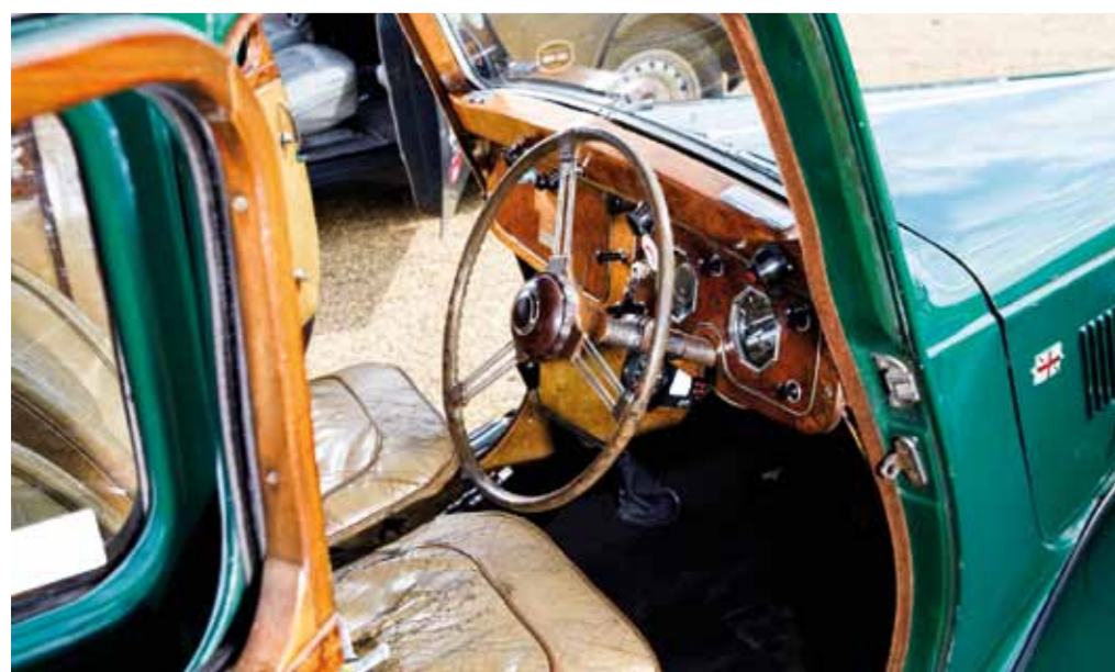
This page MG is lower and better tied-down in race trim, though it retains the cosy interior of the standard car. Engine power was almost doubled for 1954, thanks to some wild engine tuning. The car now runs a milder 1953 Stage 2 spec.
