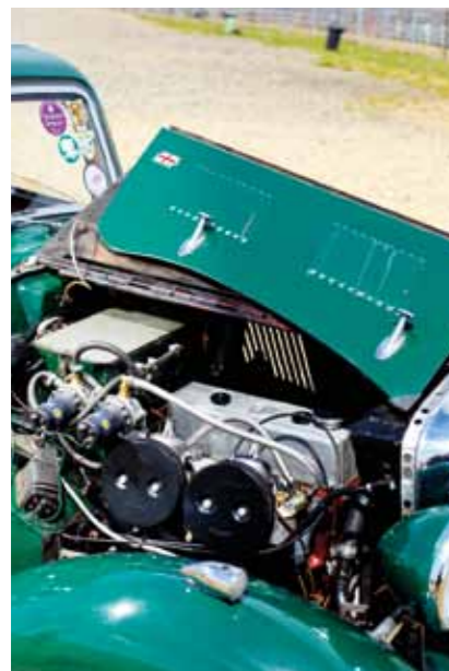
This page MG is lower and better tied-down in race trim, though it retains the cosy interior of the standard car. Engine power was almost doubled for 1954, thanks to some wild engine tuning. The car now runs a milder 1953 Stage 2 spec.
