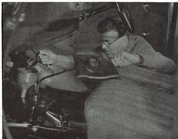
8. Fill the gearbox with the recommended grade of gear oil.
