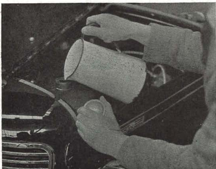
4. Check level in radiator top tank.
