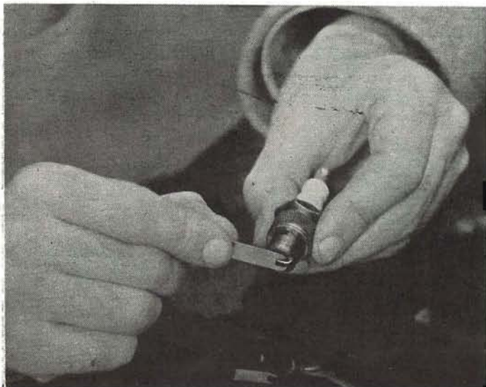
2. Sparking plug gaps should be in accordance with Instruction Manual recommendations.
