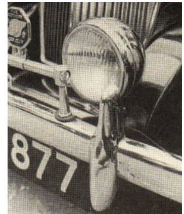
This type of fog lamp was a standard fixture and its chromium plated rear shell can be used as a rough dating clue and as an indication of originality.
