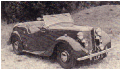
The Tourer's traditional body is based upon the ash frame of the 'Type, and its long single doors provide access via the tipping front seats to the rear seat.
