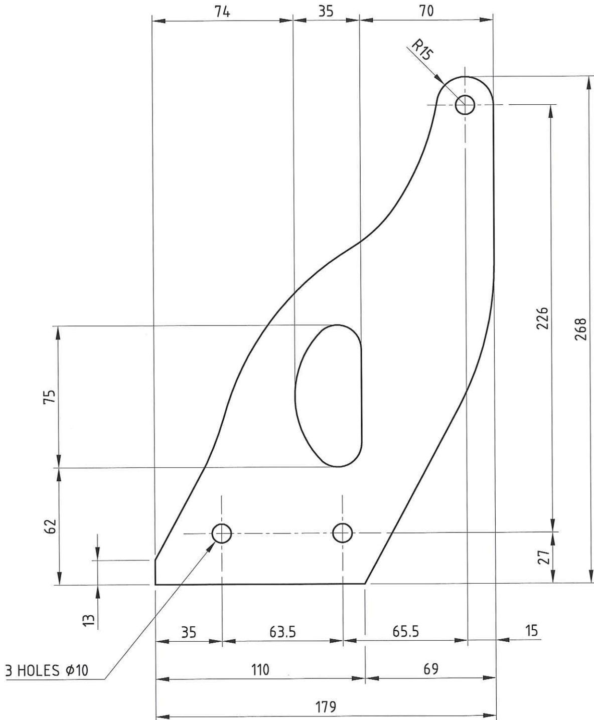
This template is designed to suit the ride height and axle location of my car. It also required modification to the bump stops and available extension of the telescopic shock absorber I used.
