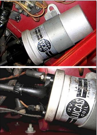
1) Coil similar to LA12: British Parts Northwest #GCL101 https://www.bpnorthwest.com/mg/mg-tc-td-tf/engineelectrical/ignition-coil-w-screw-in-ht-lead.html
