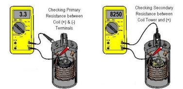
The primary resistance in an internally ballasted coil is around 1.6 ohms.
