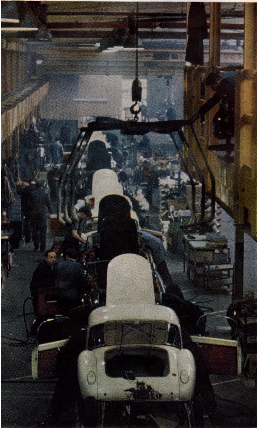
Sleek MGs move toward completion on the assembly line at the Abingdon works. The crane overhead drops a body shell onto a chassis every seven minutes. The line stops as the workers take 10-minute tea breaks at 10:20 and 4:20.
