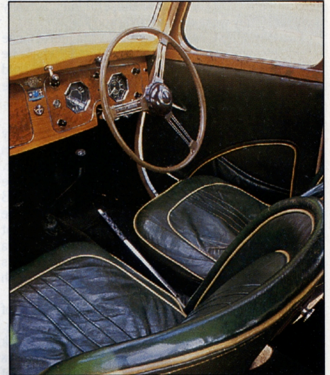
Lovely octagonal dials on 'Y' – Kimber would have approved! Front screen opens. Engine, derived from Morris Ten unit, is of 1250cc
