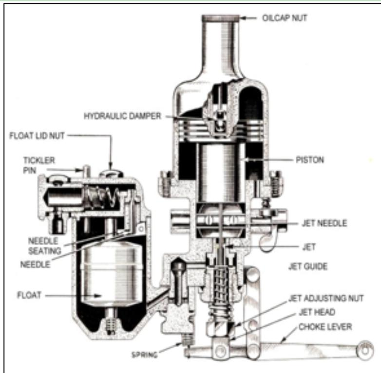
Correct setting of the float level is essential if the engine is to run well with good fuel economy. If the float level is wrong it can make starting difficult and lead to very poor mpg figures. All carburettor tuning should start with ensuring that the float level is correct.
