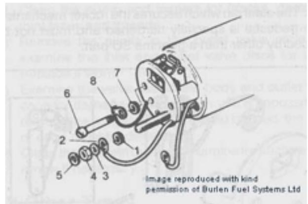
dished brass nut to the terminal screw. The correct order is shown below:
