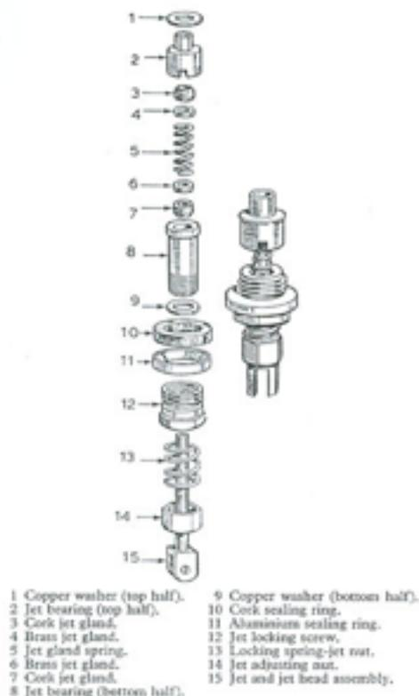
Fig. 23. H type jet components and completed assembly
