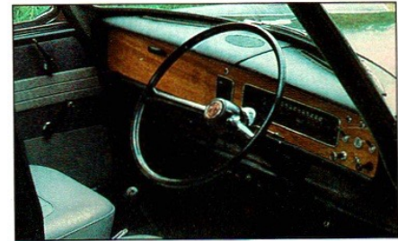
Top: B-series works hard to pull heavy Farina shell. Above: 1100 interior has strip speedo but no rev counter. Below: A-series in 1100 gives mild performance but is willing unit
