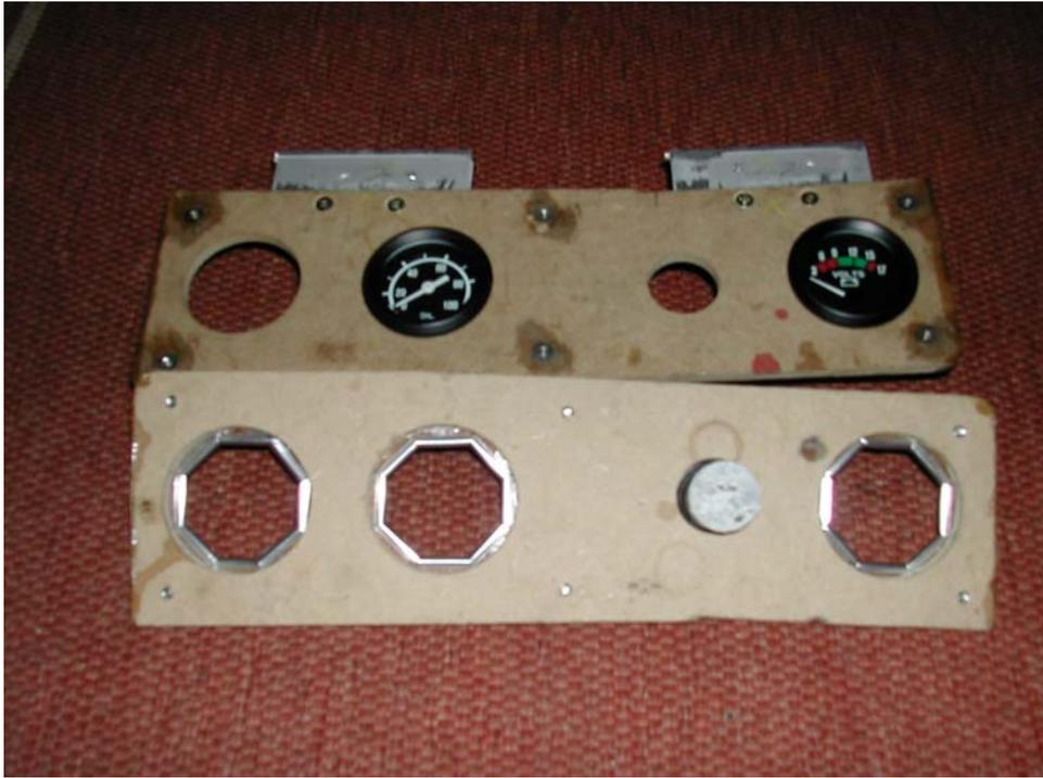
I chose to join the panels together using large headed chrome machine screws in to captive nuts in the rear panel fixed with epoxy glue, but this was largely because I already had these. I'm sure that a method of secret fixing could be devised.
