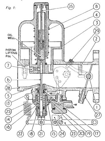
Cross sectional view of typical S.U. carb. 1: Throttle Spindle. 2: 2: Throttle Adjusting Screw. 3: Piston. 4: Suction Chamber. 5: Jet Opening. 6: Needle. 7: Needle Setscrew. 8: Piston Spring. 15: Jet Locking Screw. 18: Jet Adjusting Nut. 21: Jet Head. 22: Locking Spring. 23: Jet Lever. 24: Link. 25: Jet Return Spring. 26: Damper Rod. 28: Main Casting. 29: Fast Idle Screw.
