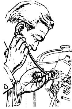
Fig. 16: Synchronization may be tested using rubber tube as stethescope, but Uni-Syn is more accurate.
