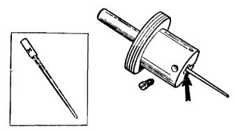
Fig. 7: Needle shoulder must be flush with piston face (arrow) except under certain conditions explained in text. Identification symbol is on shank (inset).
