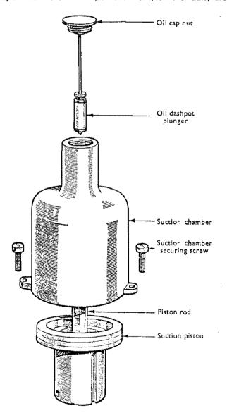
Fig. 5: The suction chamber assembly. Some models have no plunger (damper) under oil cap.
