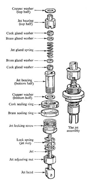
Fig 20: The Jet Assembly
