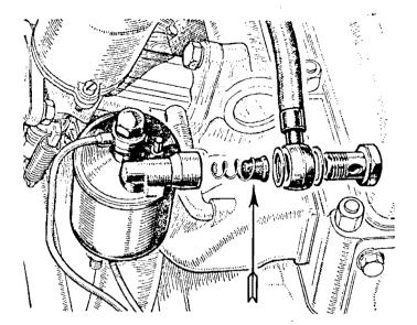
Fig. 3: To remove float chamber lid, detach fuel hose as shown, remove bolt intop of lid. Filter (arrow) must be cleaned.
