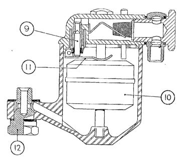
Fig. 2: The float chamber. 9: Needle Valve. 10: Float. 11: Float Lever. 12: Mounting Bolt.
