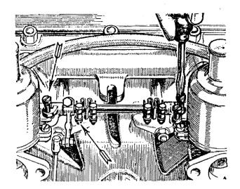
Fig. 15: Synchronization & idling speed are adjusted by screws ahown at screwdriver & upper left arrow. Spindle clamp at lower arrow must be loosened prior to synchronization. (TD shown).
