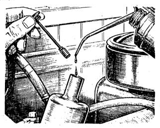
Fig. 9: Fill piston rod to within 1/2 in. of top with SAE 20 oil.
