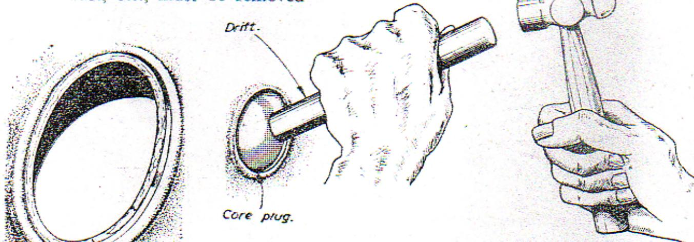
A little gasket cement is applied to the core seating.
