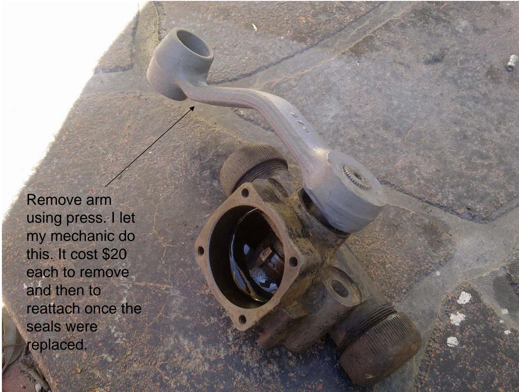
Remove arm using press. I let my mechanic do this. It cost \$20 each to remove and then to reattach once the seals were replaced.
