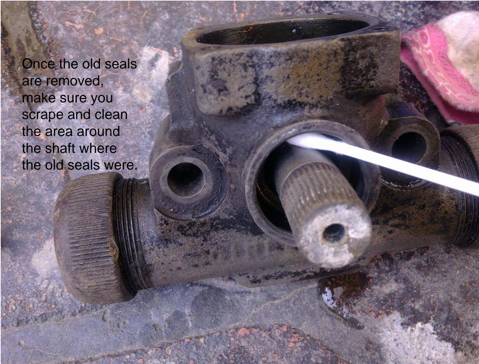
Before you insert the new seals, place two turns of masking tape around the grooves of the shaft to prevent damage to the seal. These edges are sharp and can cut into the lip of the seal which will result in oil leaking out.
