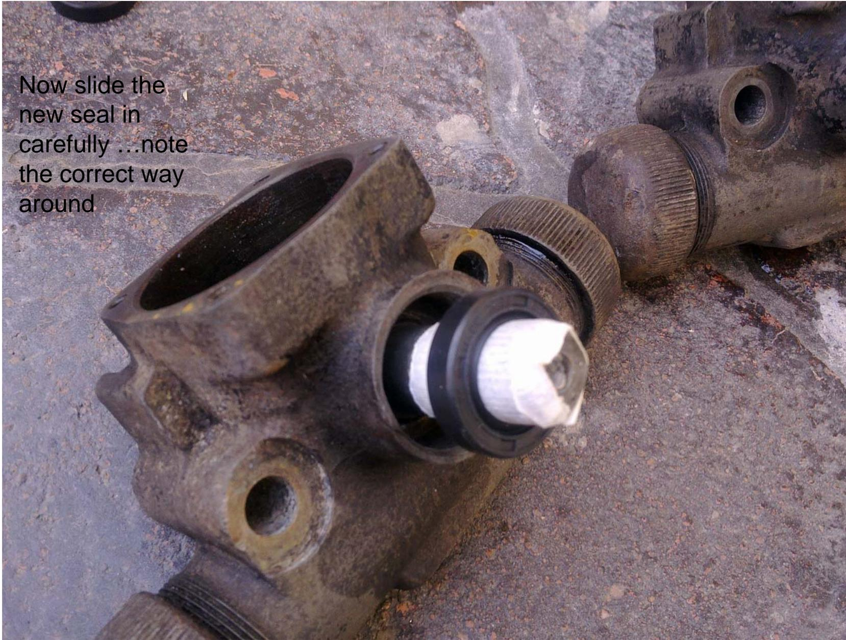
I used a spark plug socket to push it further into the damper.
