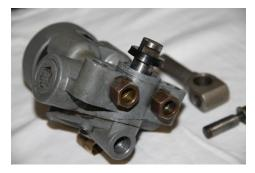
and rotate the seal around the shaft with just a little forward pressure. Then push the seal forward until it is in the cotter pin groove.
