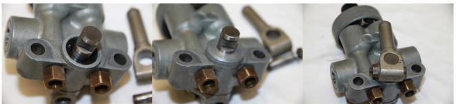
Fit the dust cover and the lever spigot together with its cotter pin. Make sure the cotter pin is firmly in place and the nut is tight. Note the cotter pin only goes into it's hole one way because it is tapered! Job done!!!
