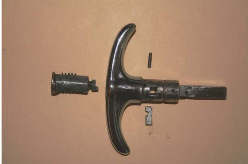
After the small retaining pin is removed, the lock cylinder should come out of the handle. My whole lock was put through a chrome plating process by the previous owner of my car, 20 or 30 years ago, and as a result the cylinder it was well and truly stuck in the handle. (I will explain how I got it out later).
