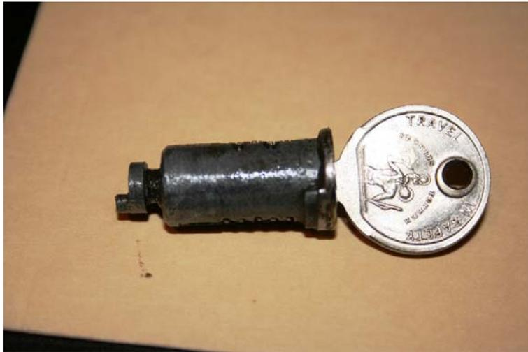
The off centre pin on the end of the cylinder pushes the small locking bar into a slot in the door lock escutcheon and when the key is removed, the door is locked.
