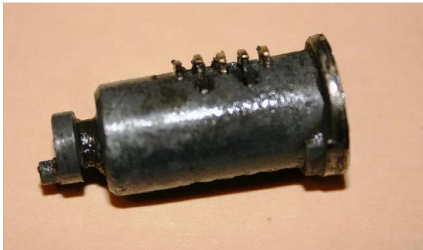
When the correct key is inserted into the lock, all the plungers disappear into the body of the cylinder, enabling the cylinder to be rotated inside the handle.
