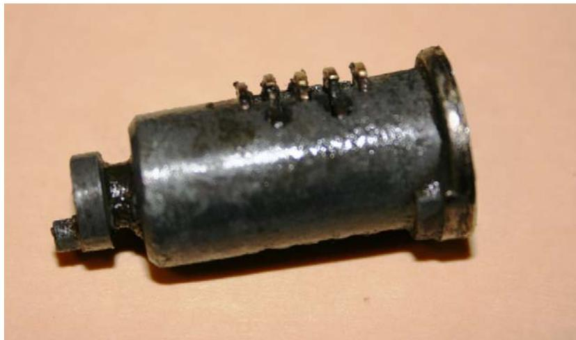
When the correct key is inserted into the lock, all the plungers disappear into the body of the cylinder, enabling the cylinder to be rotated inside the handle.
