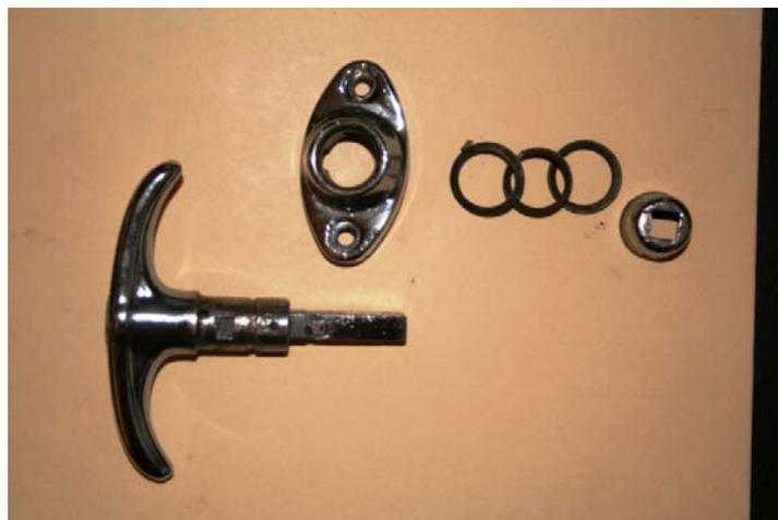
Underneath the cap is a spring with two shaped washers, one on each side of the spring. Having removed the cap, we can now access two small pins – one to hold the shaft into the handle assembly, and the second to hold the lock cylinder in place. At this point we only want to remove the lock cylinder.
