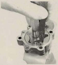
.... and between the outer rotor and the pump body. Also check that the inner rotor is secure on its shaft and the condition of the spiines or gearwheel by which the shaft is driven.
