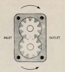
The gear type pump comprises a driving gear and a driven gear within a closely fitting housing. As the gears revolve a vacuum is created on the inlet side and oil is drawn into the pump to be carried around the perimeter of the gears and forced out of the outlet side.
