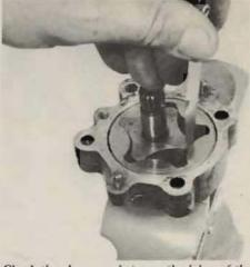
Check the clearance between the lobes of the inner and outer rotors with the rotors in the position shown . . . .
