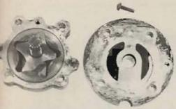
This is an eccentric vane (Hobourn-Eaton) pump with the top plate removed. The plate itself can become scored and worn and may need skimming to restore a perfectly flat inner surface. On re-assembly both the plate and the pump body faces must be perfectly clean so as to form a metal to metal seal with neither gasket not jointing compound. This type of pump was used on 'A' series engines.
