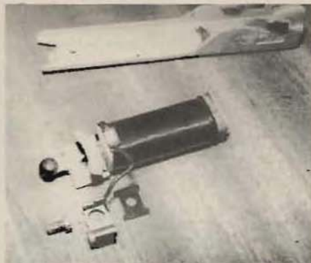
Make sure you know how the insulators are positioned under the screw which locates the solenoid and connector.
