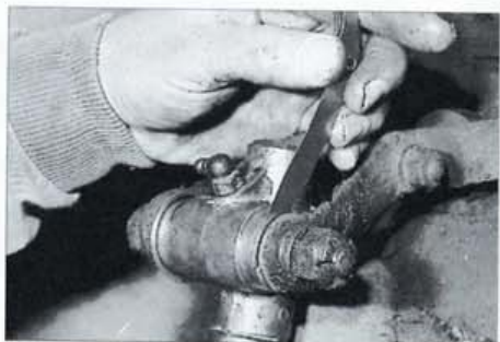
9 There must be .008in. - .013in. clearance between the trunnions and thrust washers when fulcrum bolt is fully tightened. Seals omitted for clarity.
