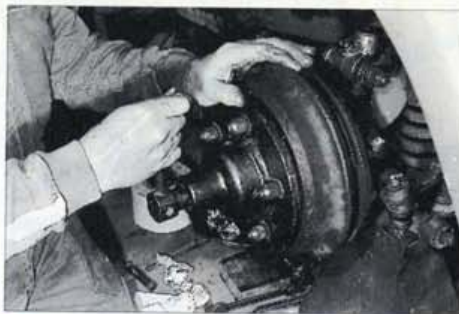
2 Using a puller to remove the hub; don't forget to slacken the adjusters first and to uncouple the brake hose and steering tie rod.
