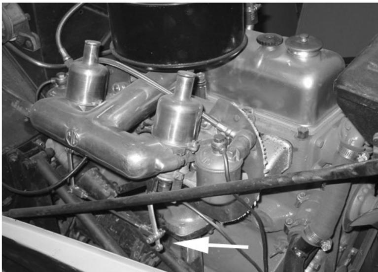
*Heat shield with carburetors and linkage in place*
