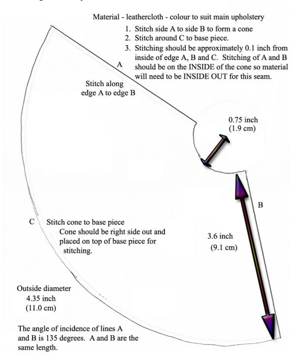
NB. This is NOT a template, but a measured drawing. Do not use this to draw around but rather as an indication for measurements. Picture for illustration purposes only.
