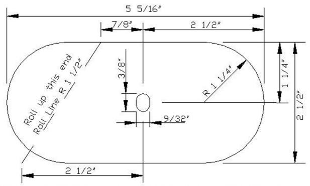
Cover Plate for Gearbox Dipstick Cut from 20SWG sheet steel Set-out is for underside
