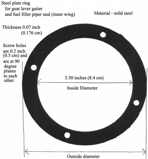
NB. This is NOT a template, but a measured drawing. Do not use this to draw around but rather as an indication for measurements. Picture for illustration purposes only.
