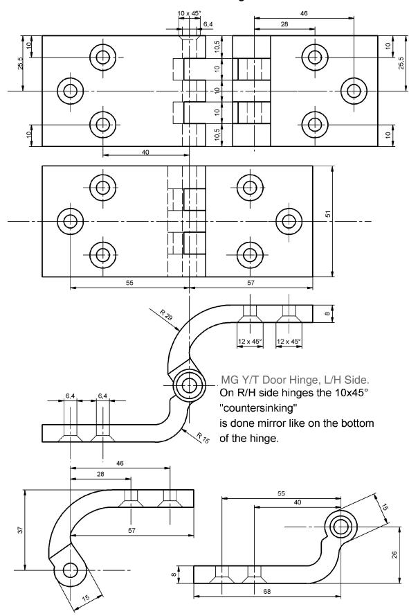
NB – This drawing does not include the chamfer that needs to but cut onto the angled inner edge of the hinge to match the curved sides of the car's body because this would have necessitated 4 drawings. One can easily check these angles with the old samples. Drawing by Anton Meyer – Switzerland.
