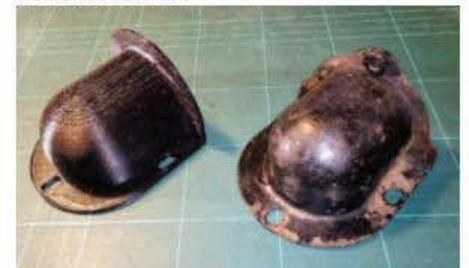
Metal end cover with 3D printed copy
