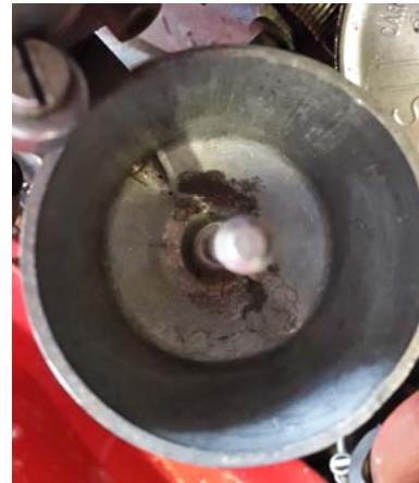
Corrosion in float chamber
