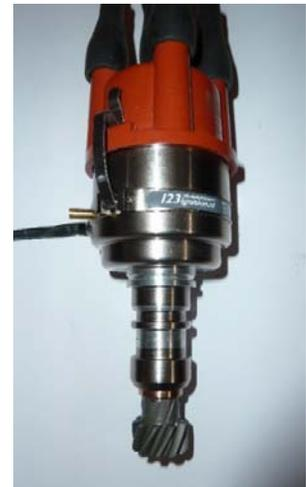
CSI also produce electronic distributor for the XPAG, however, the version with the vacuum advance has a pod similar to a mechanical distributor making fitting difficult.
