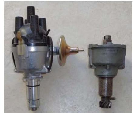
These will fit directly into later TDs and TFs (i.e. those fitted with the D2A4 distributor). However, they will require additional machining modifications in order to fit the earlier XPAG engines using a DKY4A unit. With this distributor distance between the base of the distributor and the drive gear must be increased by approximately 5mm, to accommodate the thickness of the Vernier, and a groove must be machined into the shaft to take the locating bolt.
