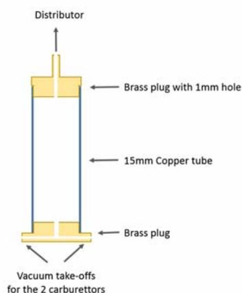
The articles on the Manchester tests have already discussed how *Slow Combustion* can result in pressure pulses in the inlet manifold. A vacuum take-off point which gives a good response to the changes in pressure, will potentially also pick up these pressure pulses and produce the wrong vacuum advance.
