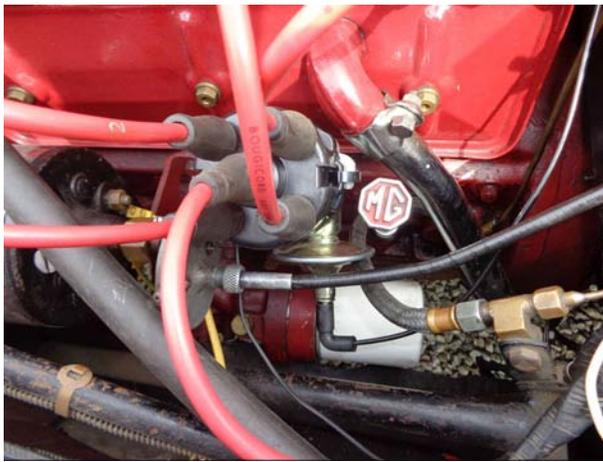
Barrie Jones has fitted a 45D4 distributor to his 1500TF. This has a relatively small vacuum pod which means it fits reasonably well in the confined space. He has used the holes in the carburettor, described below, for the vacuum take off.
