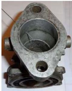
the ones fitted to later vehicles. These are normally blanked off but Burlen Fuel Systems sell an adapter that will screw into this hole. The advantage of using this is that it provides a rapid response to changes in inlet manifold pressure, hence it is advisable to consider a damper. At tick over, the hole is blocked by the butterfly which helps prevent over advancing the engine on initial pickup. If it is available, this is probably the best take off point to use with a mechanical distributor.
