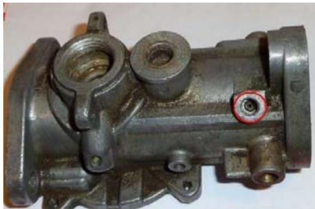
Some carburettor bodies already have a hole drilled into them at the bottom, particularly
