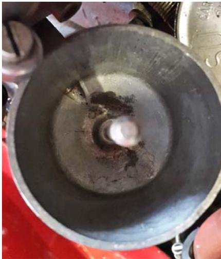
The problem also shows itself in real life. This picture shows similar corrosion inside one of my float chambers, probably caused by water getting in through the tickler pin when driving in the wet. You can see the dark line about 12 o'clock on the bottom of the chamber caused by the corrosion. When I first looked into the float chamber, there was what looked like a worm, sitting underneath the petrol at that point. This was almost certainly a small quantity of water.
