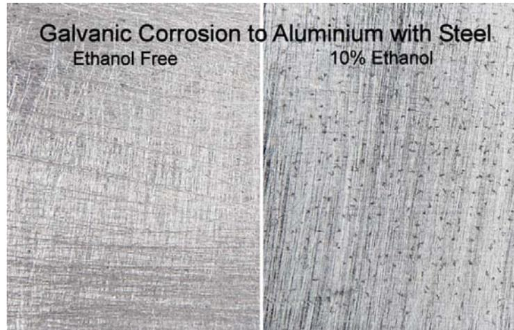
The black dots on the right hand picture are galvanic corrosion pits.
