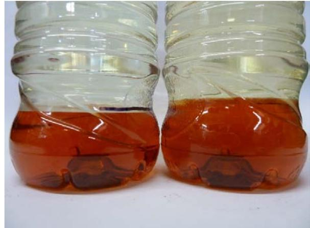
The two bottles in the picture were filled to the same level with red / brown dyed water, the petrol on the left does not contain ethanol and the one on the right does. The difference in height of the water is easy to see. (Note there is nothing at the bottom of the bottle, this is just an effect of the light on the indentation).
