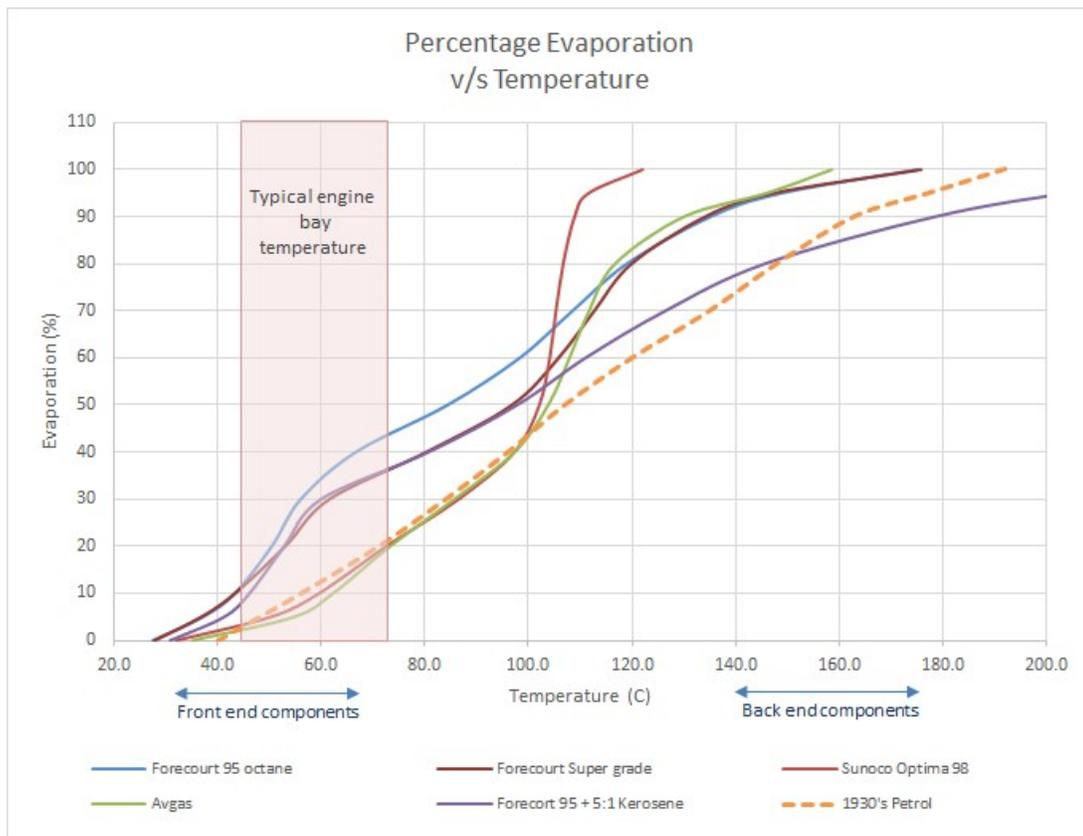
Fuels with lower front end components are less likely to suffer from the Hot Restart or Overheating problems, additionally, the test engine at Manchester also ran better on these fuels reducing the amount of waste heat produced.
