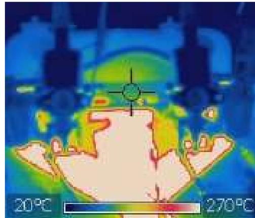
The 20°C to 42°C carburettors and float chambers, shown blue, are silhouetted against the white (300°C plus) exhaust manifold. You can also see the pipe, also blue, that links the two carburettors looping over the top of the very hot exhaust manifold.
