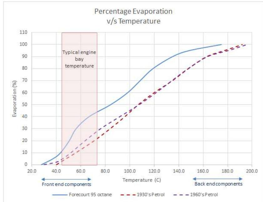
With over 40% of modern petrol evaporating at typical under bonnet temperatures, it is surprising classic carburetted engines manage to run at all. Carburettors can only deliver the correct mixture when running on liquid petrol.
