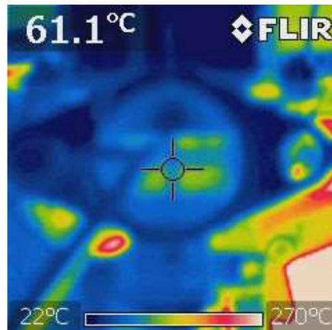
This finding is not what would be expected and explains why the thermal insulation, mentioned above, had no effect. On the XPAG the reason why the carburettors get hot after the engine has been stopped is not because of their proximity to the inlet manifold but because the hot gasses escaping back up the inlet manifold.
