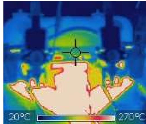
The 20°C to 42°C carburetors and float chambers, shown blue, are silhouetted against the white (300°C plus) exhaust manifold. You can also see the pipe, also blue, that links the two carburetors looping over the top of the very hot exhaust manifold.
