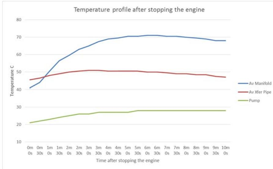
Three readings are the fuel pump (green), average of the two transfer pipes between the float chamber and carburettor (red) and the average of the temperature of the junction between the inlet manifold and carburettor (blue). As can be seen, the temperature increases of the pump outlet and transfer pipe were small.
