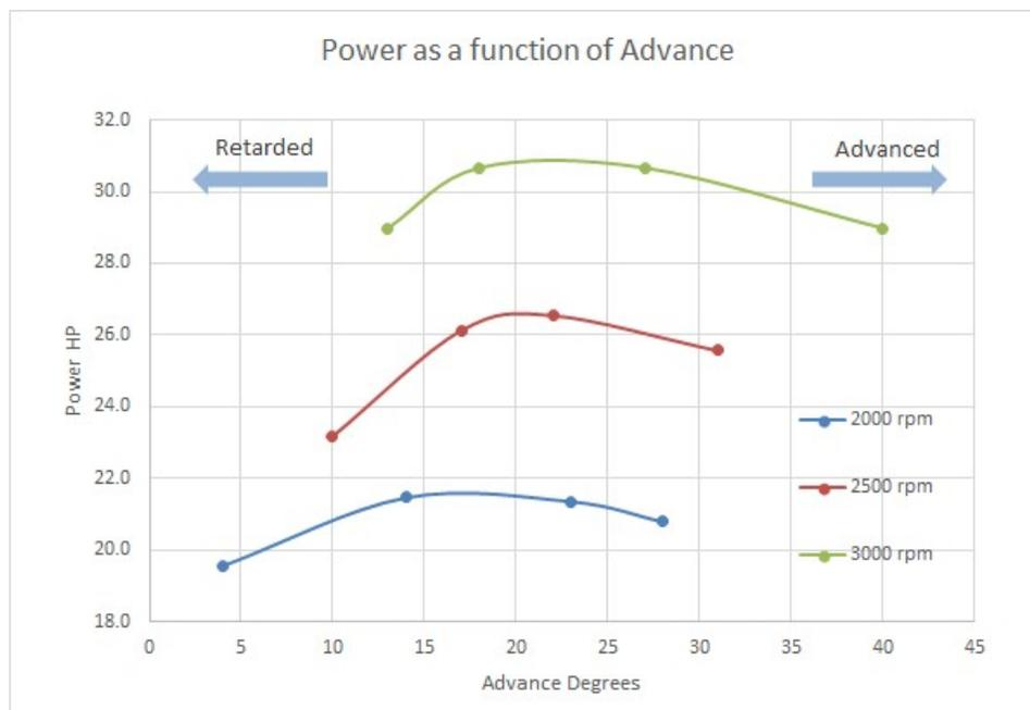
What is interesting is the insensitivity of power output to ignition timing. At 3000rpm, advancing or retarding the ignition by as much as 10-15 degrees only changed the power output by ~5%. This suggests the combustion profile is very spread as is discussed below.
