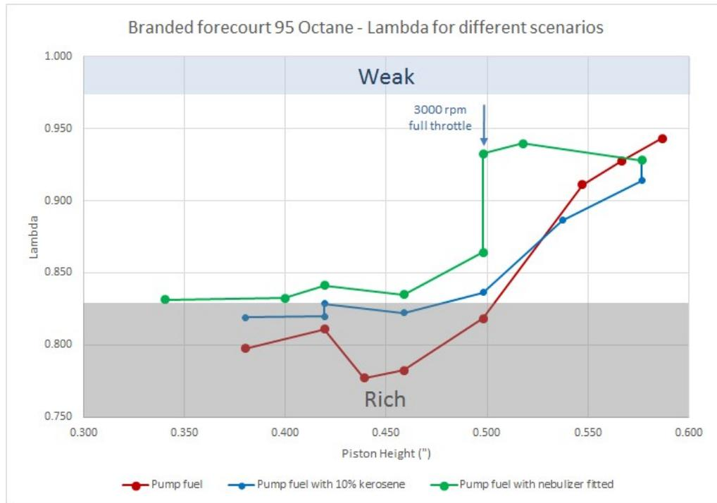
What can be seen is that, below 3000rpm, the enrichment caused by slow combustion is significantly reduced by the nebulizer (green line) and by the addition of kerosene (blue line) compared to the tests with the 95 octane petrol alone (red line).
