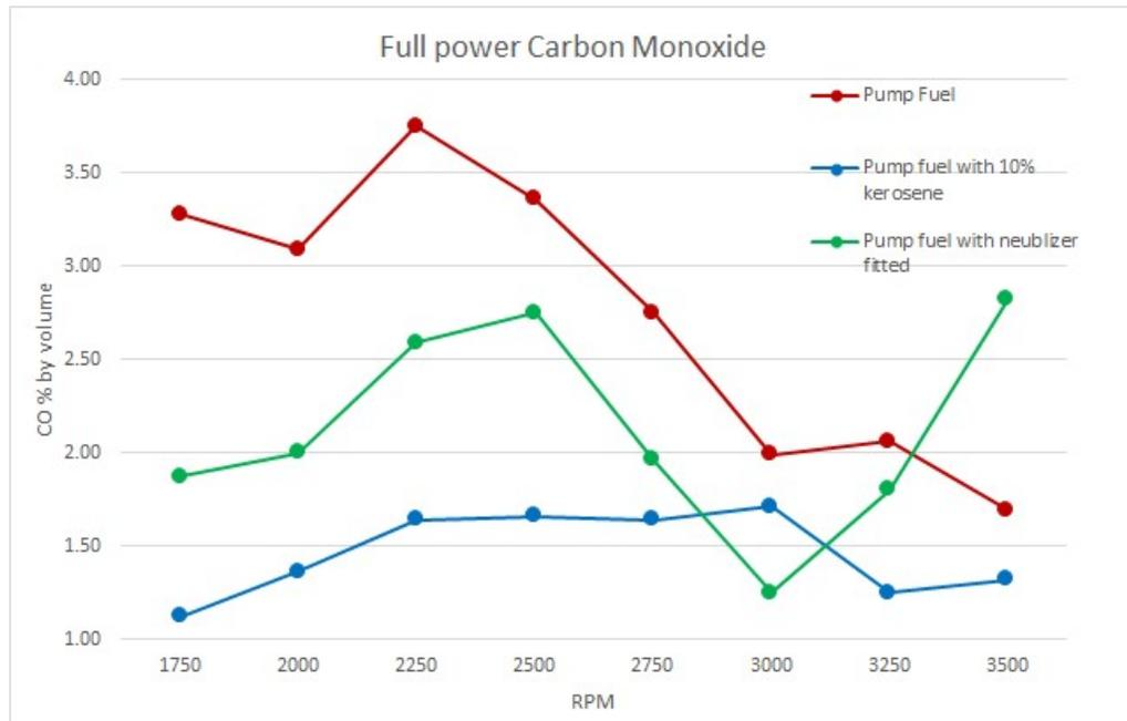
Again, below 3000rpm, the results are striking. The test run with the 95 octane petrol (red line) produced almost twice the level of carbon monoxide as that produced by the tests run with the same fuel but with the nebulizer and added kerosene (green and blue lines). Interestingly, this data suggests the combustion is more complete with kerosene than with the improved mixing produced by the nebulizer. I do not have an explanation for this.
