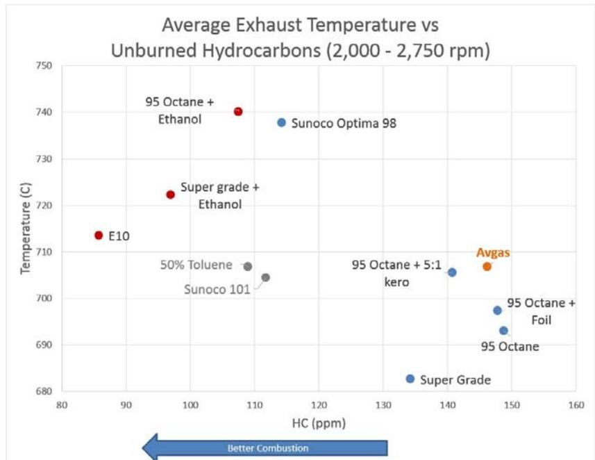
It is interesting to note at the bottom right hand of the graph, the 95 Octane + foil and 95 Octane + 5:1 kero both burn better than the 95 Octane on its own. Adding kerosene certainly improves the combustion suggesting any fears it will not burn are unfounded.
