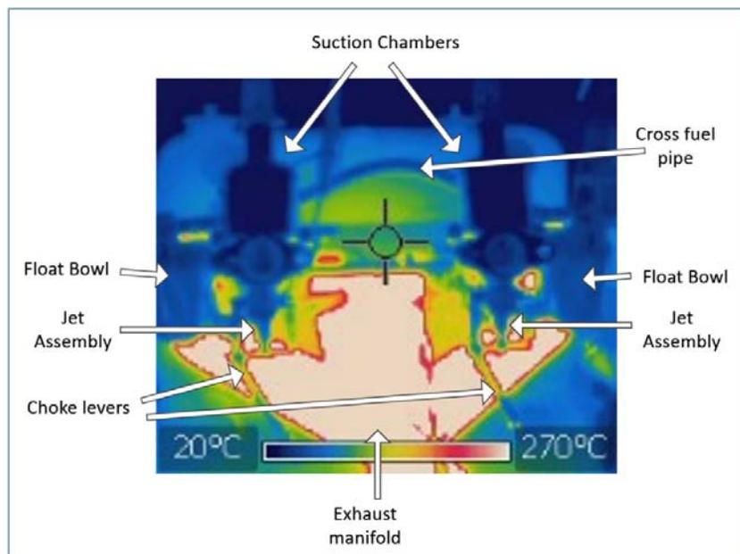
One clear message from the Manchester tests was that it was not obvious which parts of the fuel system get hot. For example, the thermal camera images showed the float bowls to be relatively cool, even though they were close to the inlet manifold whilst the choke levers were surprisingly hot.
