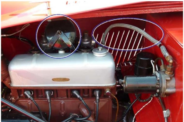
Although I do not suffer from the hot restart problem, when switching on the ignition after a short stop, the petrol pump will sometimes continue to click as it tries to pump against the petrol vapour in the fuel pipes or cannot suck vapour from the feed pipe. This shows the potential dangers of running petrol hoses through the hotter parts of the engine bay.
