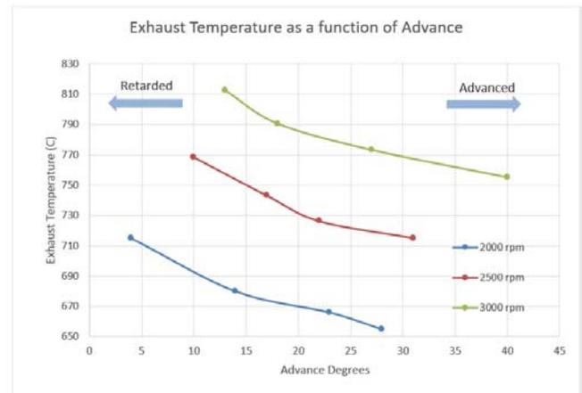
When setting the ignition timing, providing you are not experiencing pinking, it is better to err on the side of being too advanced than being too retarded. This will help reduce exhaust gas and under bonnet temperatures with only a minor loss of power.
