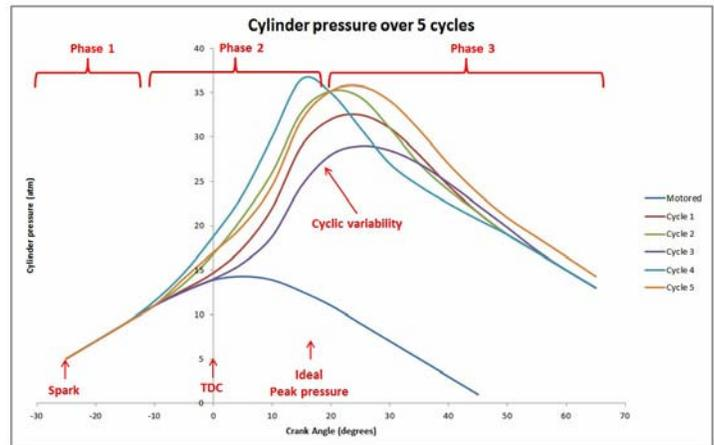
If we were to produce what is called a *peak pressure frequency plot* for these 5 cycles by counting how many cycles occurred between 15° and 19° after TDC (marked in blue below), 20° to 24° (marked in orange) and 25° to 29° (marked in green),
